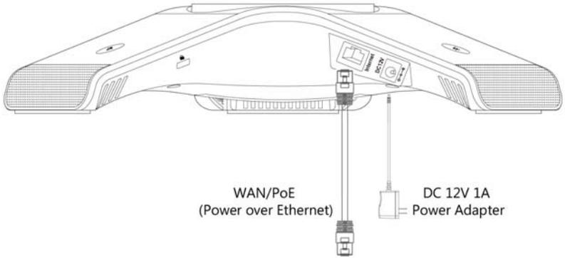
1. Connect the WAN port to the network with the provided Ethernet cable.
